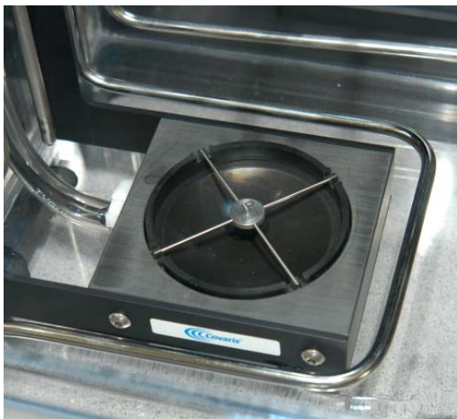
The 500141 Intensifier (left) shown installed in the E210 transducer well and (right) removed.
