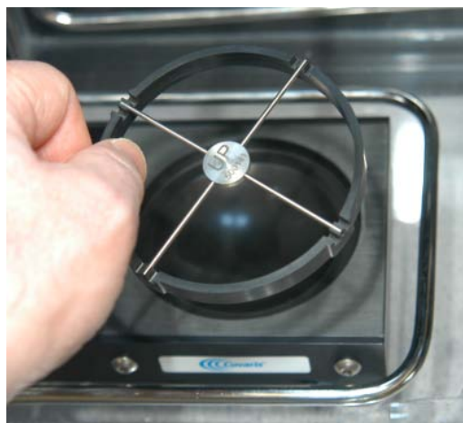
The 500141 Intensifier (left) shown installed in the E210 transducer well and (right) removed.
